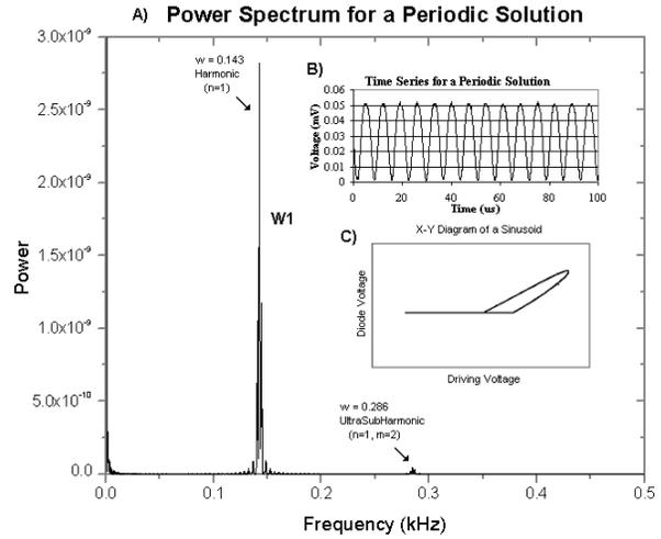
**Fig. 2:** Response of the driven diode resonator when exhibiting periodic behavior. Driven at a frequency of 143 kHz and amplitude of 50 mV. The harmonic frequency is at 143 kHz and the ultrasubharmonic is at 286 kHz ( $f/2$ ). A) Power Spectrum; B) Raw data of the diode voltage; C) Phase plot of diode voltage vs. drive voltage<sup>4</sup>.
