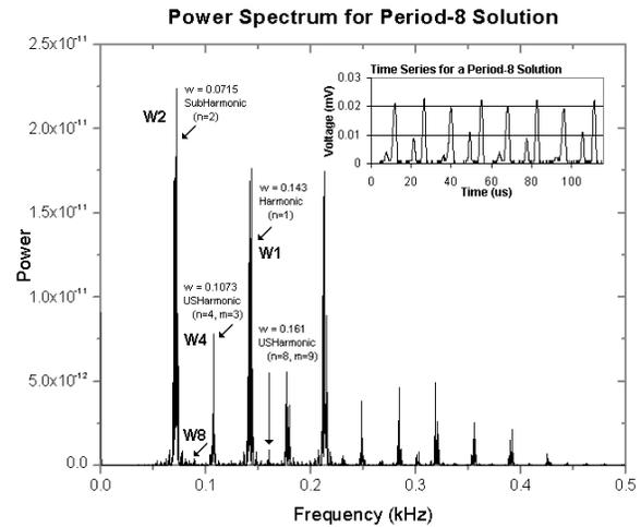
**Fig. 5:** Response of the driven diode resonator when exhibiting a period-8 solution. Driven at a frequency of 143 kHz and amplitude of 238 mV. A) Power Spectrum; B) Raw data of the diode voltage; C) Phase Plot of diode voltage vs. drive voltage<sup>4</sup>.
