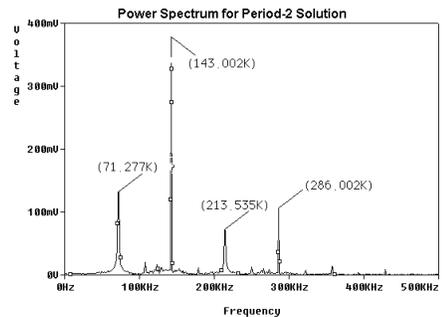
**Fig. 8:** Computer simulation of an FFT for a period-2 solution to a diode resonator circuit. The resonant frequency is found at 143 kHz and the subharmonic frequency can be seen at 71.3 kHz.
