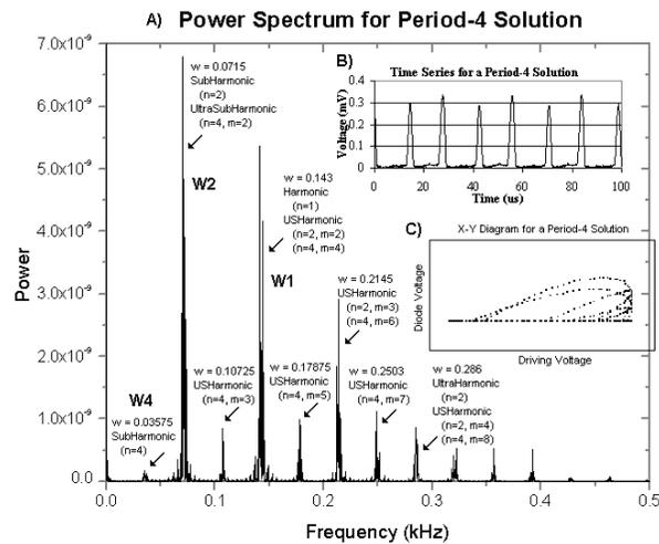
**Fig. 4:** Response of the driven diode resonator when exhibiting a period-4 solution. Driven at a frequency of 143 kHz and a voltage of 220 mV. The harmonic frequency of the system is 143 kHz and the subharmonic frequencies are at 71.5 kHz ( $f_0/2$ ) and 35.75 kHz ( $f_0/4$ ). A) Power Spectrum; B) Raw data of the diode voltage; C) Phase Plot of diode voltage vs. drive voltage<sup>4</sup>.
