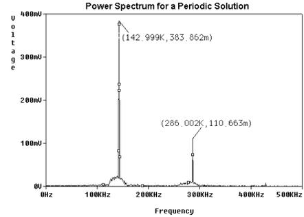
**Fig. 7:** Computer simulation of an FFT for a periodic solution to the diode resonator circuit. Resonant frequency is found at 143 kHz and an ultraharmonic frequency can be seen at 286 kHz.
