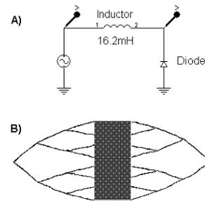
**Fig. 1:** A) Description of the diode resonator circuit. Composed of an inductor and diode in series. The voltage is measured across the inductor. B) Bifurcation diagram for the circuit. As the system approaches chaos, the periodic state will divide to a period-2 state, period-4 state, etc., until the adjoining states are too close to distinguish.
