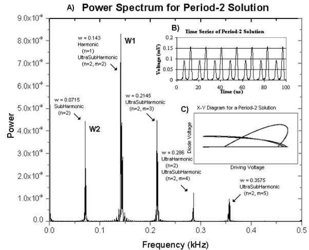
**Fig. 3:** Response of the driven diode resonator when exhibiting a period-2 solution. Driven at a frequency of 143 kHz and a voltage of 178 mV. The harmonic frequency of the system is at 143 kHz and the subharmonic frequency is 71.5 kHz ( $f/2$ ). A) Power Spectrum; B) Raw data of the diode voltage; C) Phase Plot of diode voltage vs. drive voltage<sup>4</sup>.
