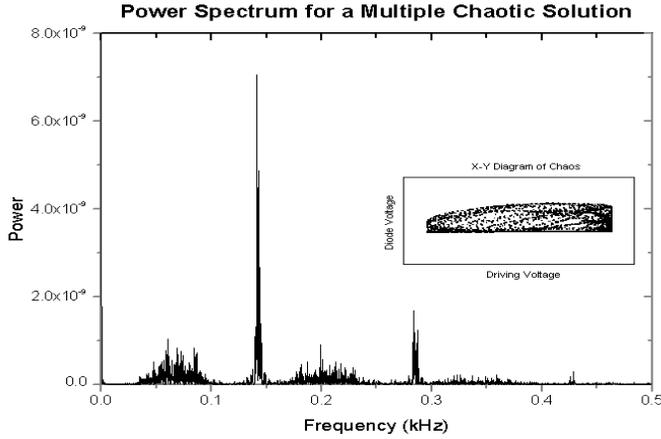
**Fig. 6:** Response of the driven diode resonator when exhibiting multiple chaotic behavior. Driven at a frequency of 143 kHz and amplitude of 304 mV. Peak frequencies are still visible at the resonant frequency 143 kHz but a wide spectrum of frequencies is seen between the harmonics.
